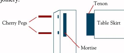
We use classic joinery techniques. All table frames are made with double-pinned mortise and tenon joinery.
